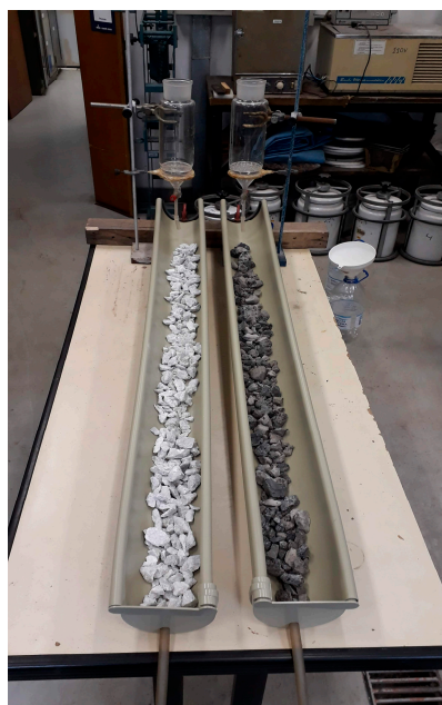
Figure 4. Acid drainage treatment experiments involving open channels with limestone ( left ) and slag ( right ) at the bench scale.
